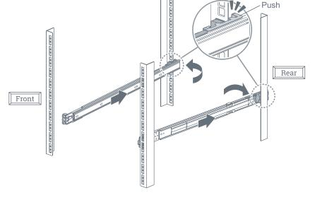
Adjust the length of the rail kit assembly, and insert the front end to the rack by slightly sliding the front latch outwards and inserting the brackets into the rack holes.
