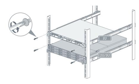
For 17-Series\* and future 2U/3U chassis, slide inwards and hold the rail kit release tabs on the ear holders, and pull out the chassis from the rack. \* Not including RS3617xs
