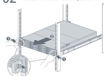
Slide outwards the rear latch of the inner rail to unlock the inner rail from the outer rail assembly. With the help of another person, carefully remove the chassis from the rack. (You may remove all HDDs first to reduce the weight of the chassis.)
