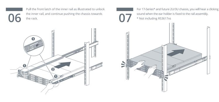
Use the cage nuts and screws in the rail kit package to secure the chassis to the rack if necessary.
