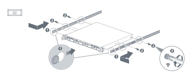
With the help of another person, carefully align the inner rails to the outer rail assembly, and push the chassis towards the rack.
